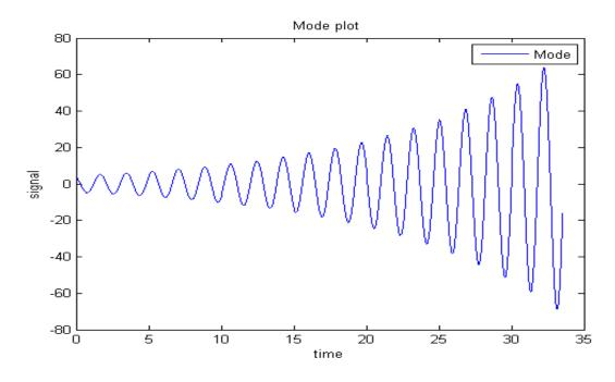
Fig 6.8: 31<sup>st</sup> July 2012: 0.55 Hz (damping: -0.2%)---post disturbance
