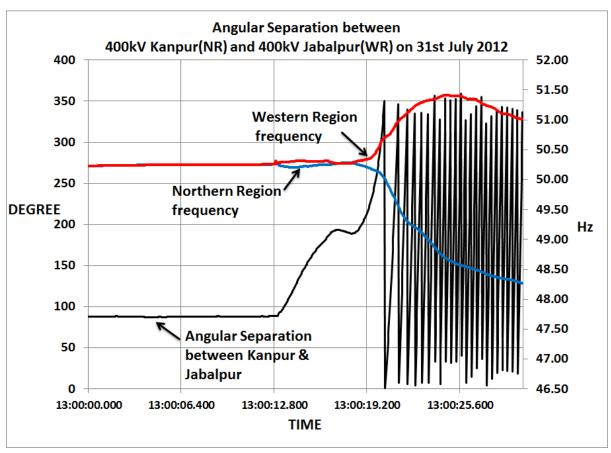
Fig 6.2: Frequency profile and angular separation from the Phasor Measurement Units (PMUs) at NRLDC
