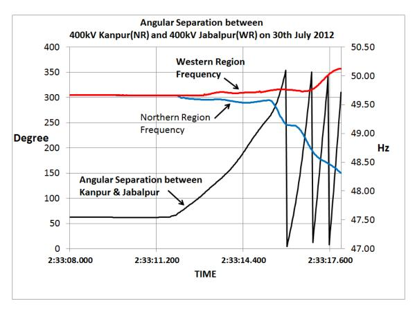
Fig 3.2: Frequency profile from the Phasor Measurement Units (PMUs) data at RLDCs
