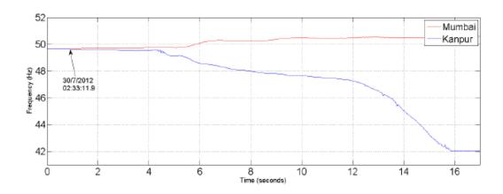
Fig 3.3: Frequency profile as captured by IIT Bombay's Wide Area Frequency Measurement System
