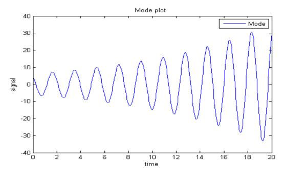
Fig 6.7: 31st July 2012—0.53 Hz (damping:-2%)-pre-disturbance
