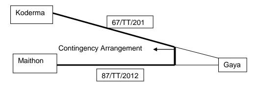
38. In the instant petition, the petitioner has mentioned to the constituents of Eastern Region that these 2 nos. 50 MVAR line reactors may be installed and commissioned as Bus reactor at Maithon Sub-Station to control the voltage problems, and these Reactors will be commissioned along with the line as a Line Reactors. The Schematic diagram is shown overleaf:-
