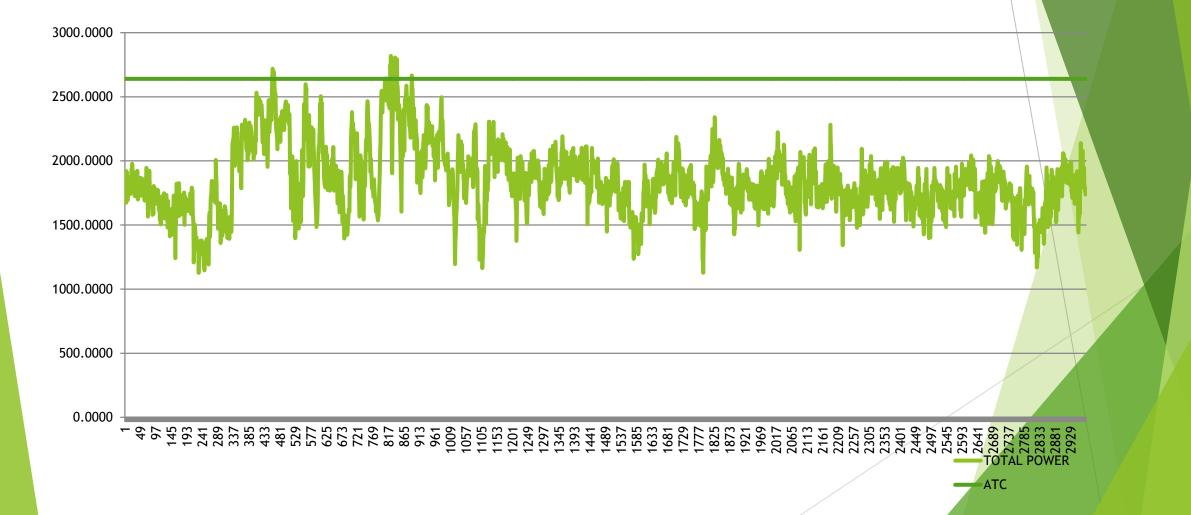
Power flow on a single circuit of 400 kV D/C Kolar-Hosur line (15 minute readings for May 2014) (critic line in S1-S2)
