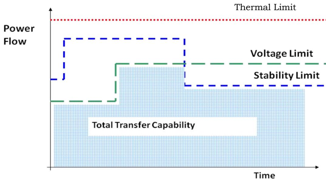
**Total Transfer Capability is the minimum of the Thermal Limit, Voltage Limit and the Stability Limit**
