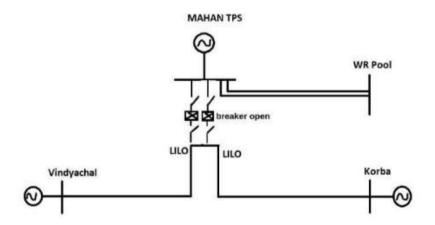
However, subsequently on analysis of the proposed scheme based on SLD obtained from EPMPL it was observed that Vindhyachal & Korba 400kV lines are terminated in two separate dia in Mahan TPS switchyard. Hence, it would not be possible to bypass the LILO line within the switchyard by keeping breakers open. To finalise the modalities of implementation of the above proposal, a separate meeting was held on 23.12.2021 amongst WRPC, CEA, CTU, POSOCO, EPTCL,
