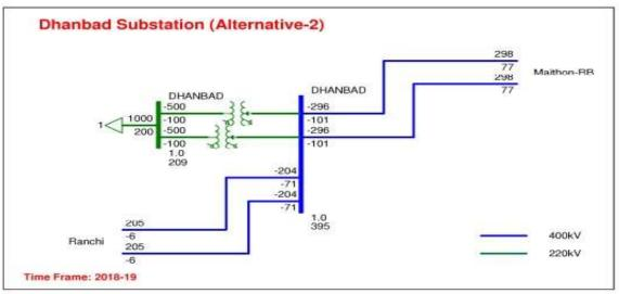
16.2 AGM, POWERGRID stated that out of the two alternatives studied, the alternative two i.e. LILO of both circuits of Ranchi-Maithon RB 400 kV D/C line at Dhanbad is more suitable.
