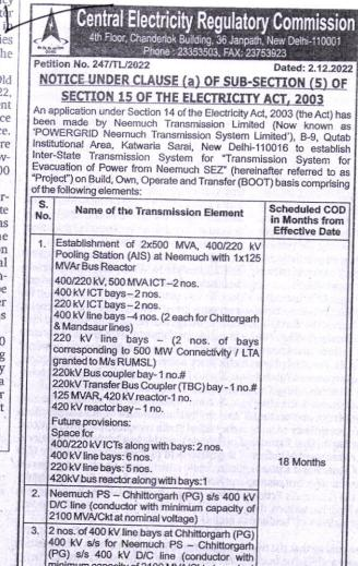
(conductor with minimum MVA/Ckt at nominal voltage) 2 no. of 400 kV line bays at Mandsaur 400 kV s/s for Neemuch PS- Mandsaur s/s 400 kV D/c line (conductor with minimum capacity of 2100 MVA/Ckt at nominal voltage)
